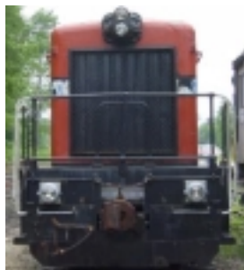
In order to be allowed to go out on the Mainline the Museums diesels had to have ditch lights and an event recorder installed per FRA standards.
